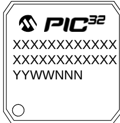
100-Lead TQFP (12x12x1 mm)
