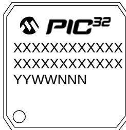
100-Lead TQFP (12x12x1 mm)
