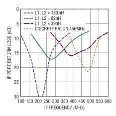
Figure 2. IF+ Port Output Return Loss
