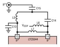
Figure 3. IF Output with Discrete IF Balun Matching
