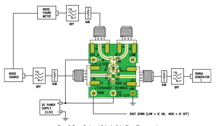
Figure 7. Proper Equipment Setup for Noise Figure Measurement
