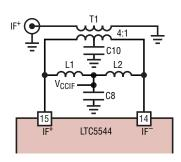
Figure 1. IF Output with Bandpass Matching
