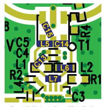
Figure 4. Modifications for Discrete IF Balun Matching
