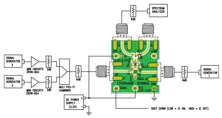
Figure 6. Proper Equipment Setup for RF Performance Measurements
