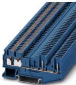
Feed-through terminal block, Connection method: Push-in / plug connection, Cross section: 0.14 mm<sup>2</sup> - 4 mm<sup>2</sup>, AWG: 26 - 12, Width: 5.2 mm, Color: blue, Mounting type: NS 35/7,5, NS 35/15
