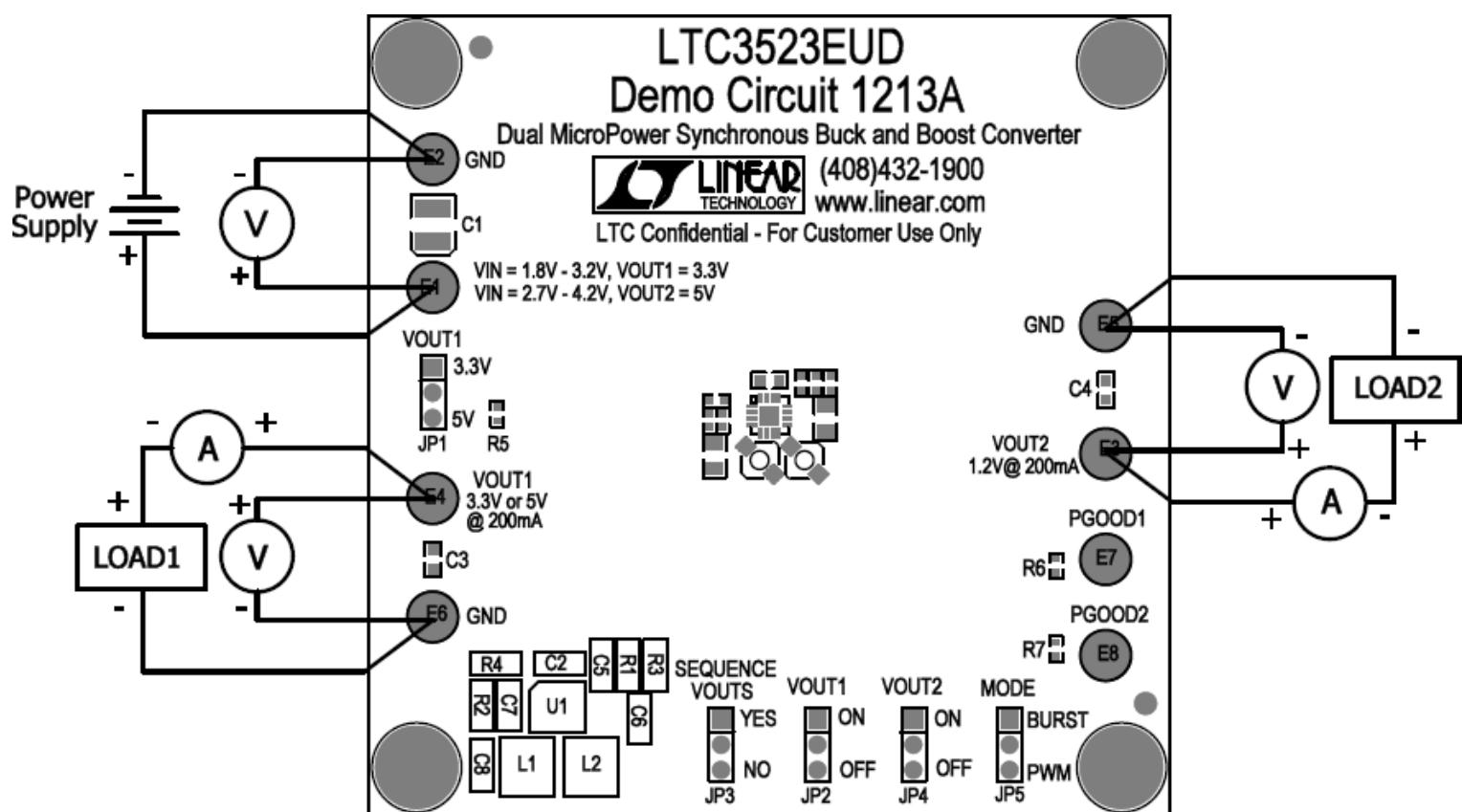
Figure 1. Proper Measurement Equipment Setup
