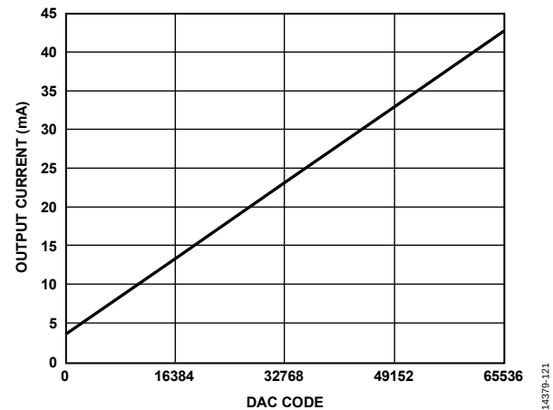
Figure 190. Gain Curve for ANA_FULL_SCALE_CURRENT[9:0] = 1023, DAC Offset = 3.8 mA
