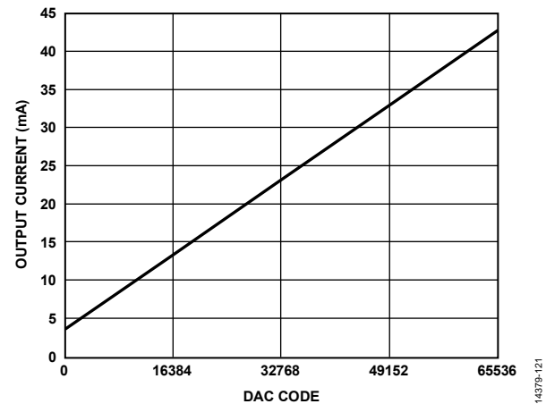
Figure 190. Gain Curve for ANA_FULL_SCALE_CURRENT[9:0] = 1023, DAC Offset = 3.8 mA
