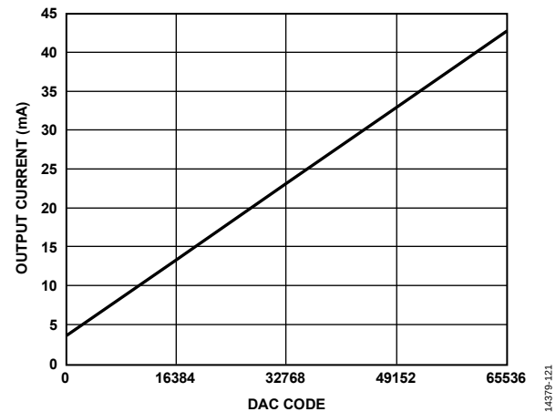
Figure 190. Gain Curve for ANA_FULL_SCALE_CURRENT[9:0] = 1023, DAC Offset = 3.8 mA
