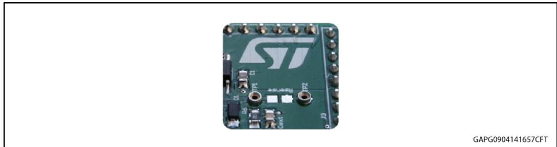
Figure 4: Mounting through-hole sense resistor
