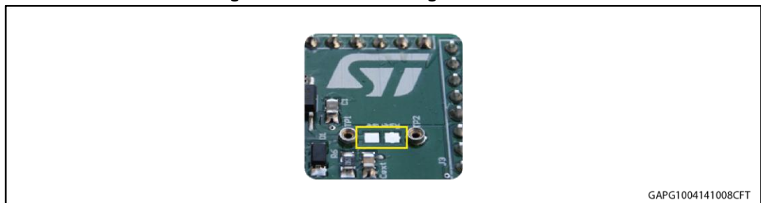
Figure 5: Pads for soldering SMD resistor
