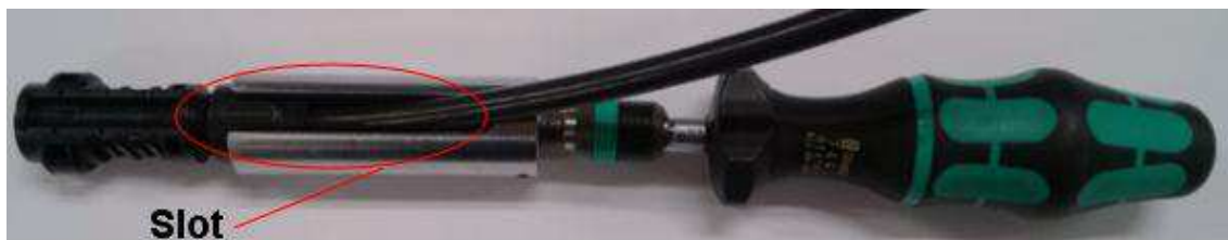
Figure 9 Tightening of the cable screw joint nut
