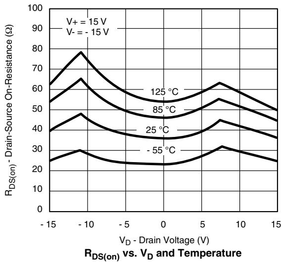
**$R_{DS(on)}$  vs.  $V_D$  and Temperature**
