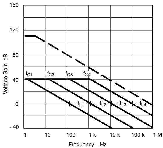
$$A_L \text{ (Voltage Gain Below Break Frequency)} = \frac{R_3}{R_1} = 100 \text{ (40 dB)}$$
