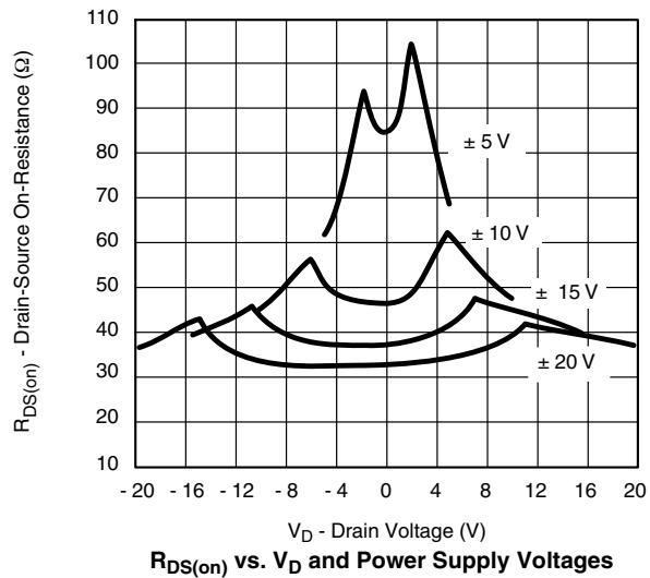
**$R_{DS(on)}$  vs.  $V_D$  and Power Supply Voltages**
