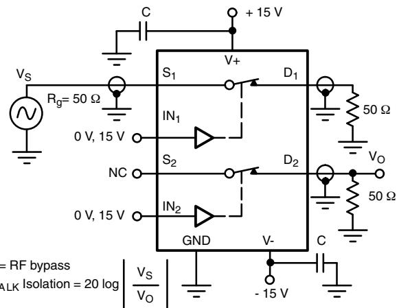
**Figure 4. Channel-to-Channel Crosstalk**
