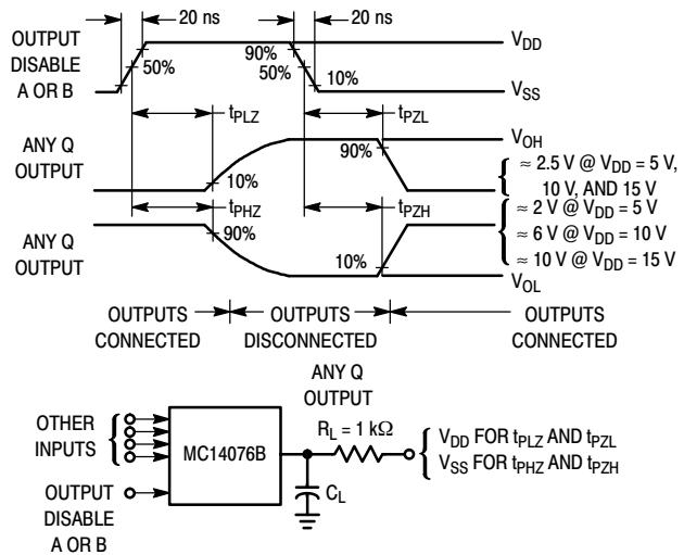
Figure 2. Three-State Propagation Delay Waveshape and Circuit
