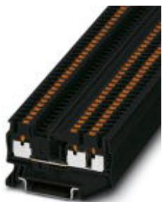
Feed-through terminal block, Connection method: Push-in connection, Cross section: 0.14 mm<sup>2</sup> - 4 mm<sup>2</sup>, AWG: 26 - 12, Width: 5.2 mm, Color: black, Mounting type: NS 35/7,5, NS 35/15
