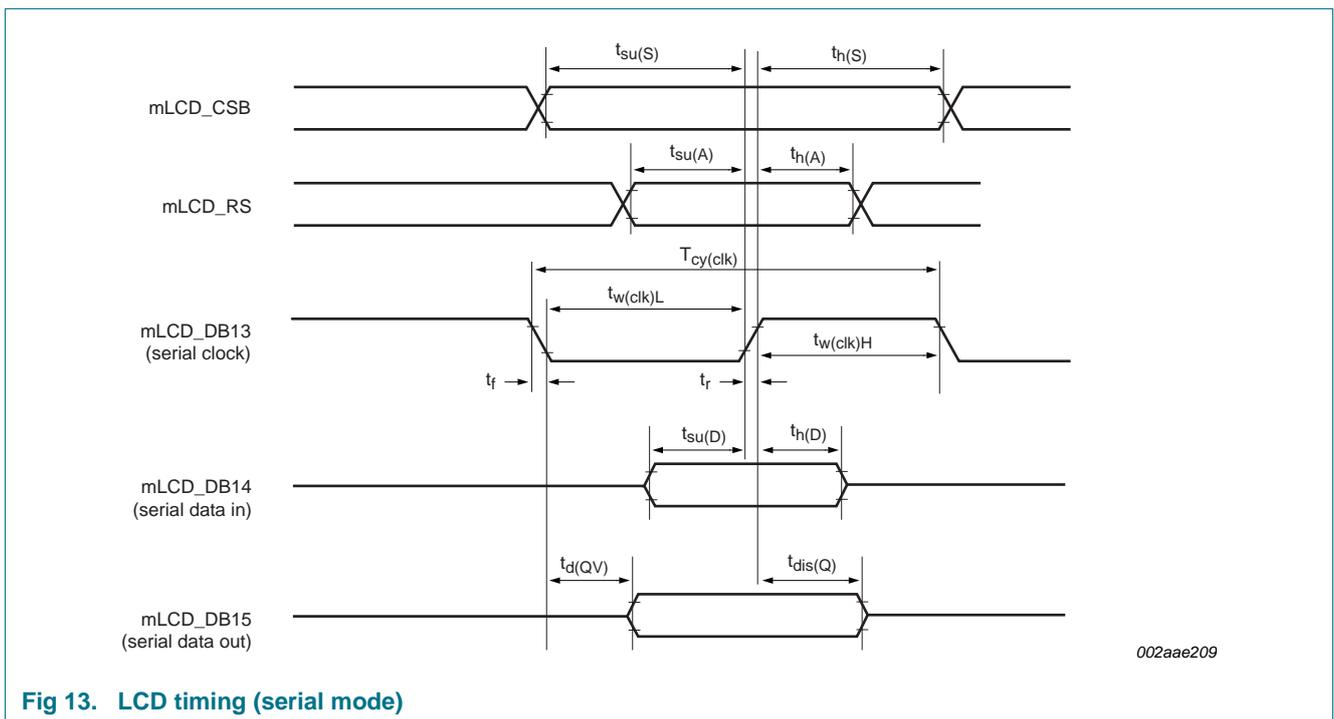
Fig 13. LCD timing (serial mode)
