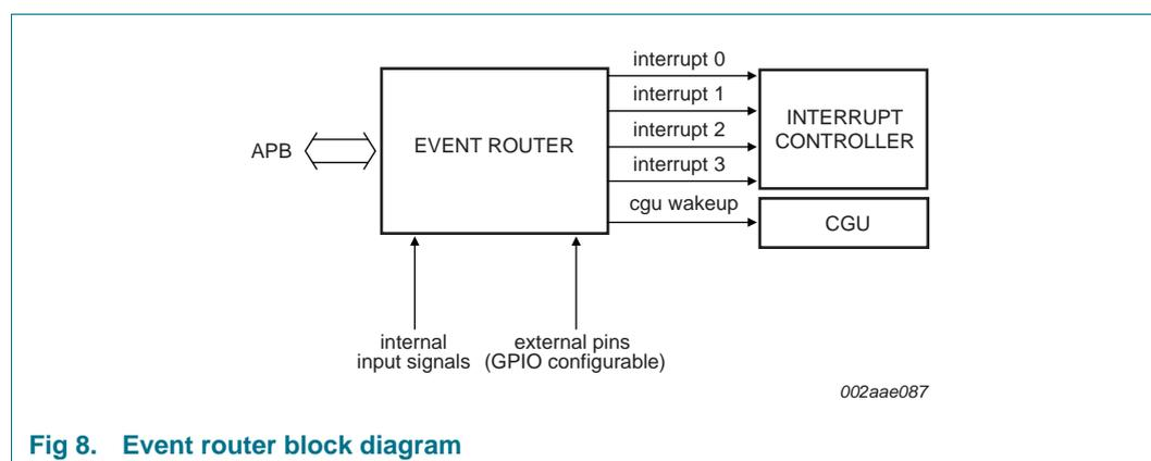
**Fig 8. Event router block diagram**
