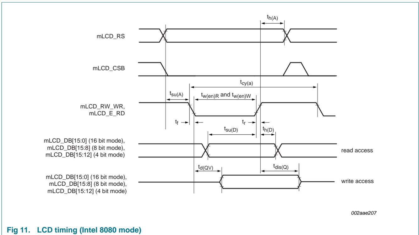
**Fig 11. LCD timing (Intel 8080 mode)**
