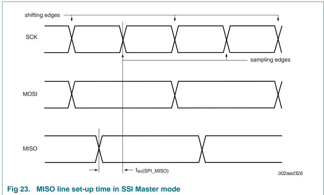
Fig 23. MISO line set-up time in SSI Master mode
