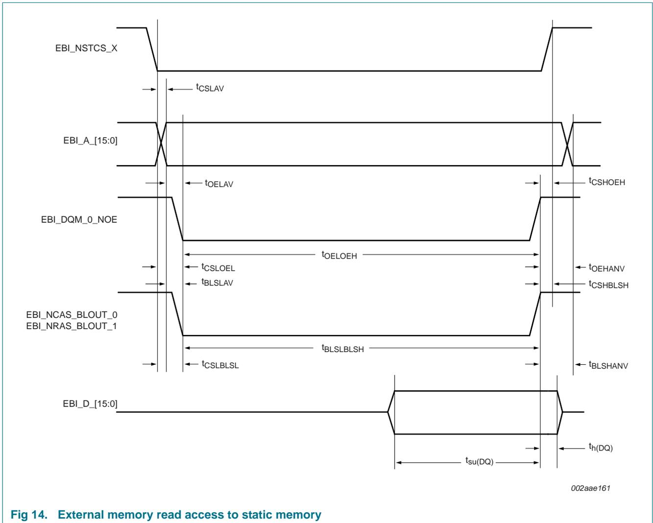
Fig 14. External memory read access to static memory
