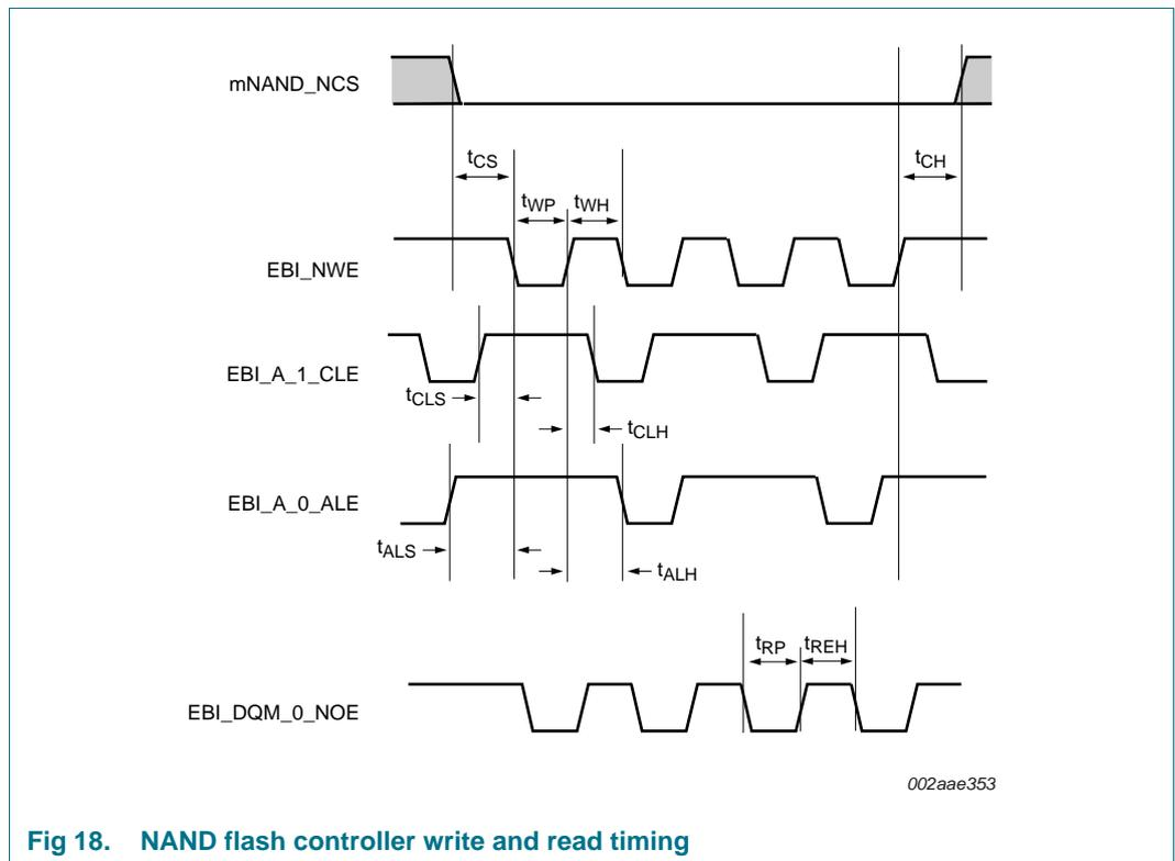
**Fig 18. NAND flash controller write and read timing**
