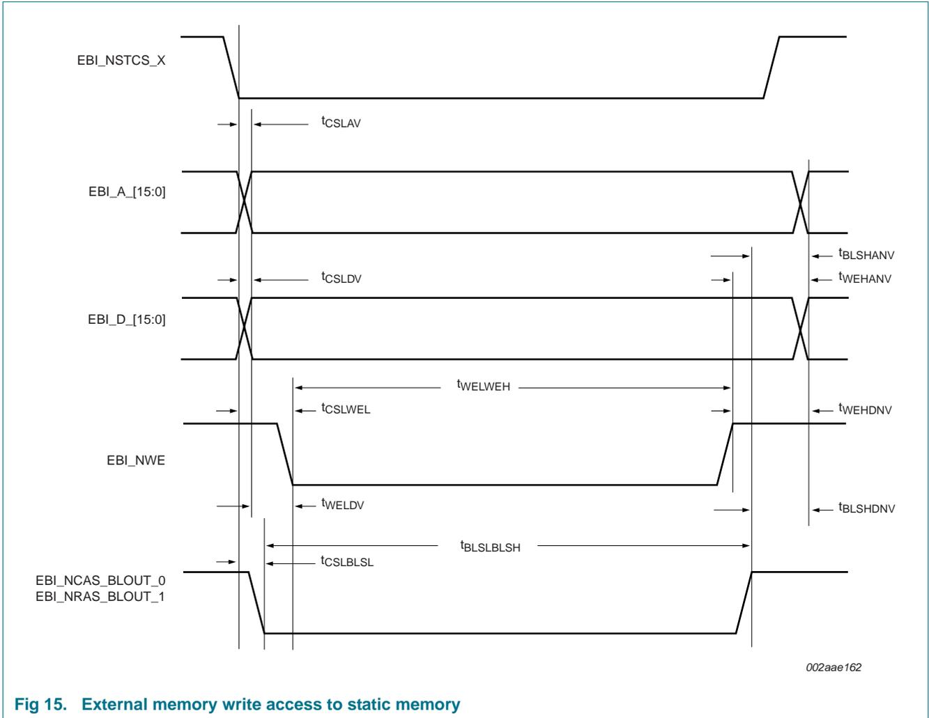
Fig 15. External memory write access to static memory
