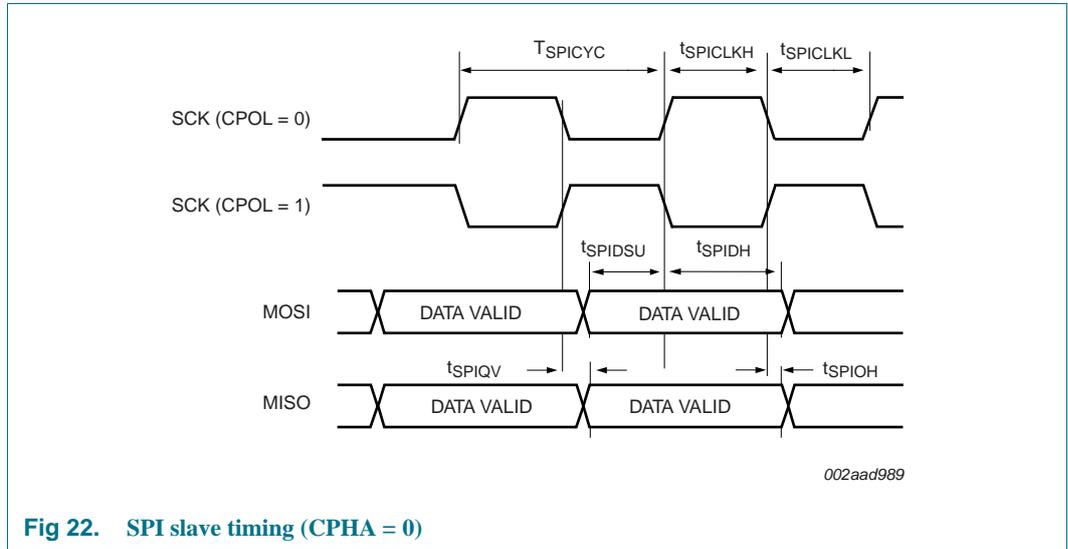
Fig 22. SPI slave timing (CPHA = 0)
