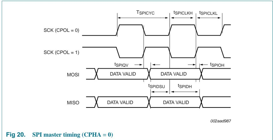
Fig 20. SPI master timing (CPHA = 0)
