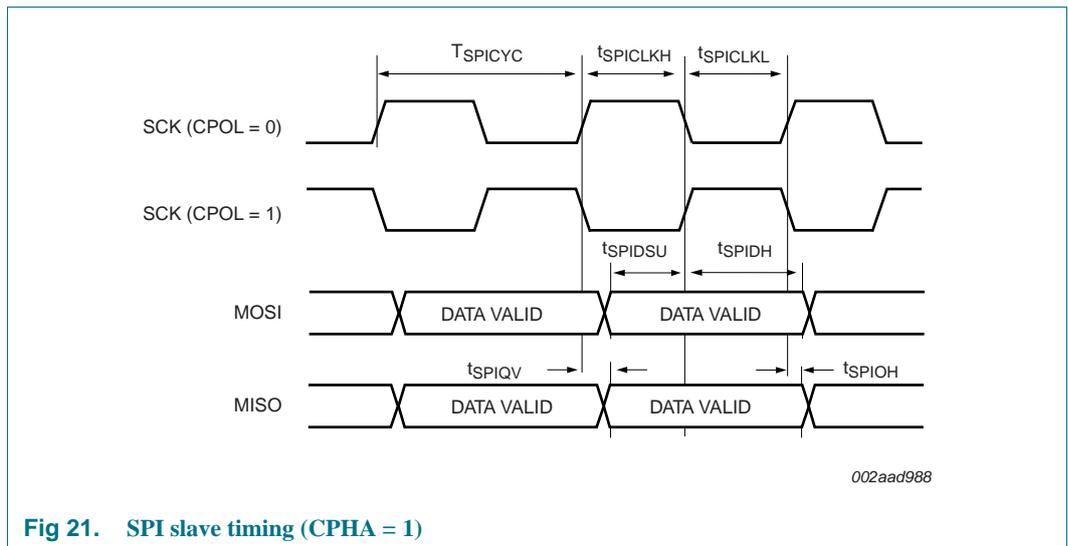
Fig 21. SPI slave timing (CPHA = 1)
