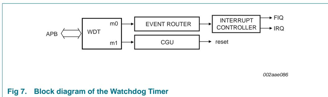
Fig 7. Block diagram of the Watchdog Timer
