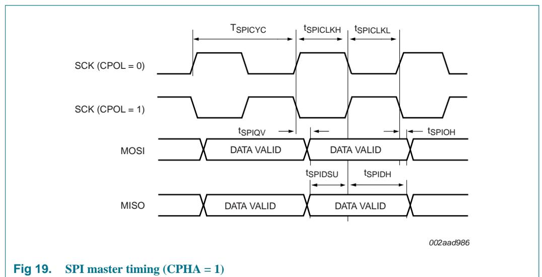
Fig 19. SPI master timing (CPHA = 1)
