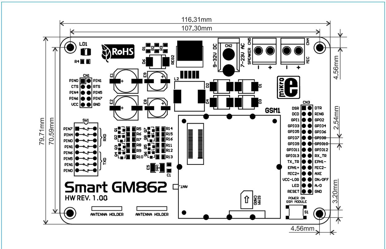
Figure 3: SmartGM862 dimensions
