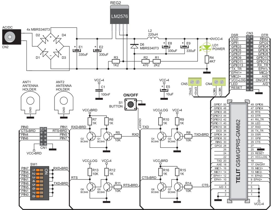
Figure 4: SmartGM862 connection schematics
