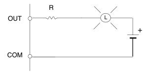
Transistor Output Residual Voltage
