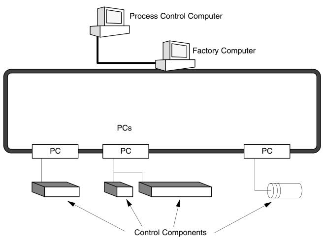
A Control System can involve very large applications where many different models of PC are networked together or it could be an application as small as a single PC controlling a single output device.
