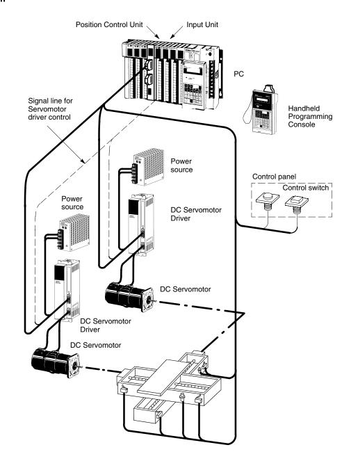
In the typical Control System example shown above, a PC controls the movement of the workpiece bed across two horizontal axes using Limit Switches and Servomotors to monitor and control movement.
