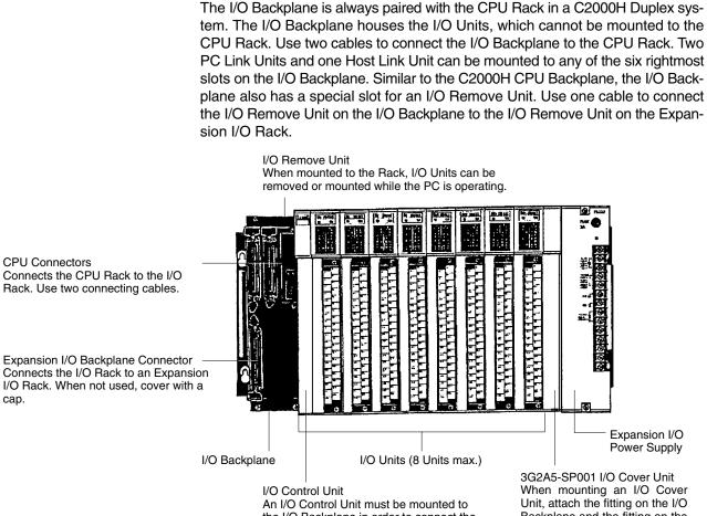
the I/O Backplane in order to connect the I/O Backplane to Expansion I/O Racks.
