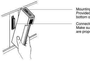
Mounting screws Provided at the top and bottom of the Unit
