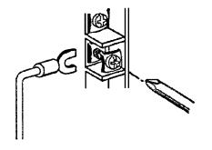
Use ring crimp terminals for wiring. Do not connect bare stranded wires directly to terminal blocks.
