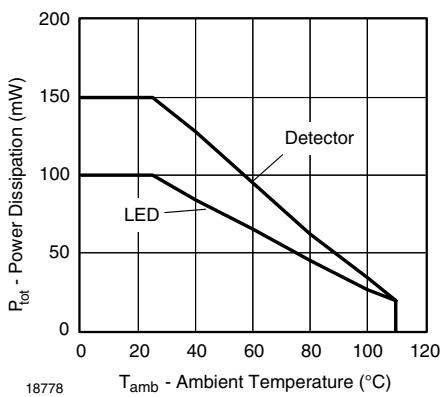
Fig. 1 - Permissible Power Dissipation vs. Ambient Temperature
