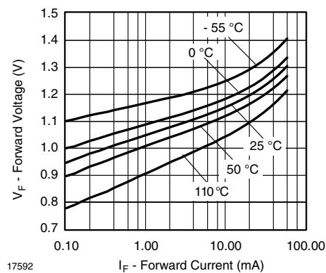
Fig. 2 - Forward Voltage vs. Forward Current
