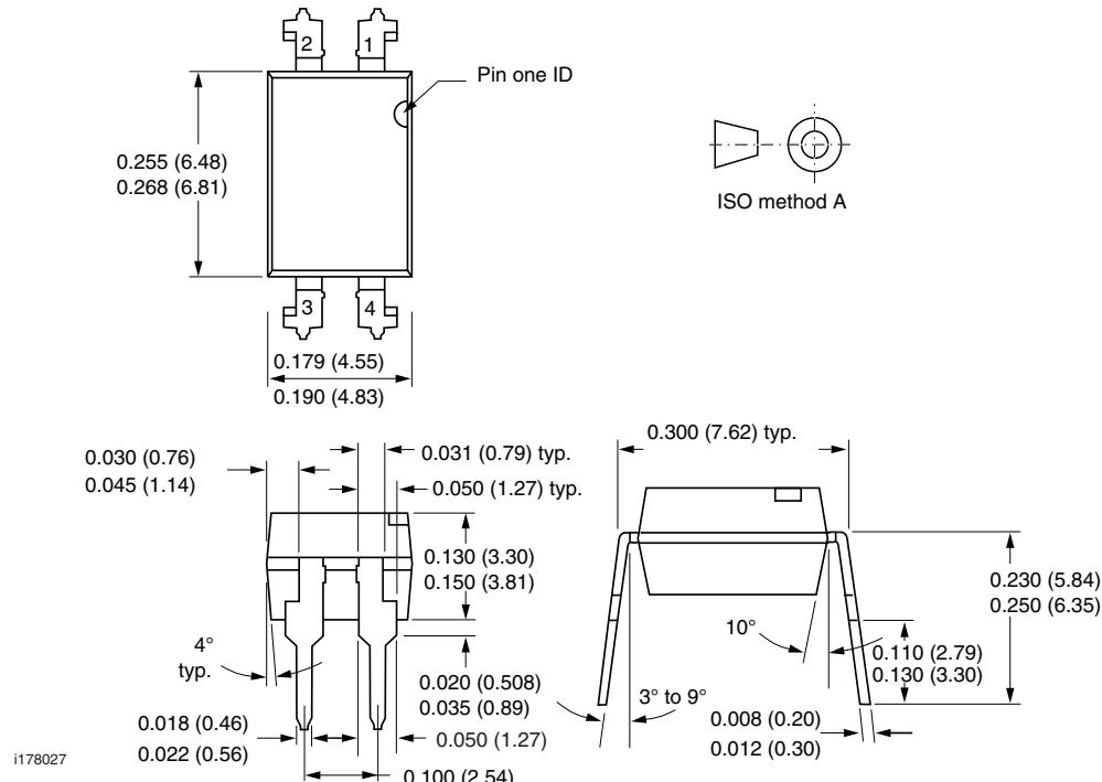
Vishay Semiconductors      Optocoupler, Phototransistor Output,
