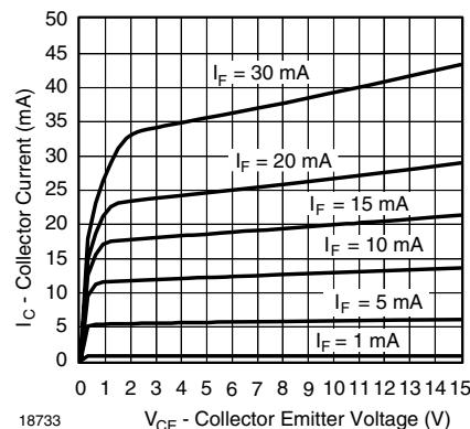
Fig. 3 - Collector Current vs. Collector Emitter Voltage
