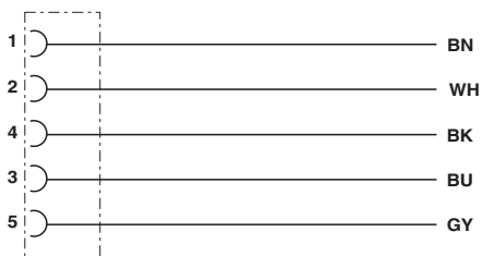
Contact assignment of the M12 socket
