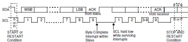
**Figure 80: Data transfer on the I2C Bus**
