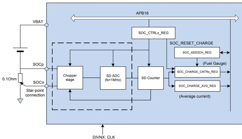
Figure 22: State of charge (SOC) circuit block diagram
