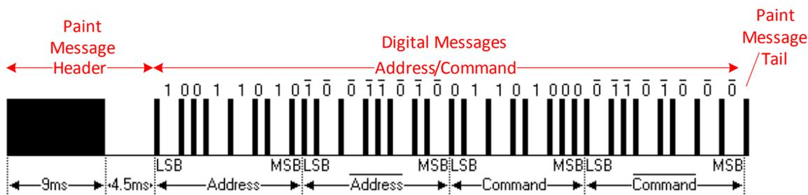
Figure 90: Paint/Digital messages on a NEC based example
