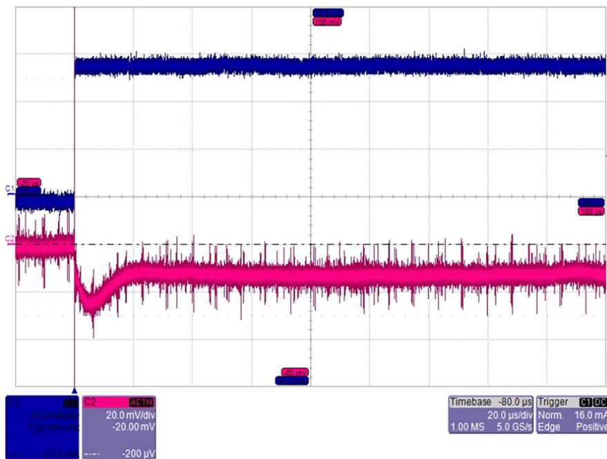
Figure 14: LDO\_IO loadstep 0 to 60mA (Cload=10uF)
