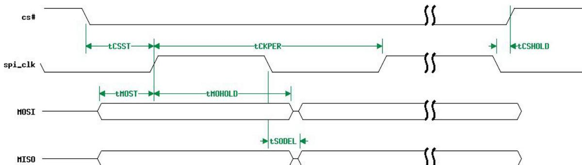
Figure 77: SPI slave mode timing (CPOL=0, CPHA=0)
