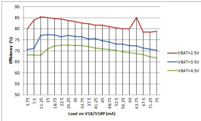
Figure 10: 1.8V rails DCDC efficiency vs load
