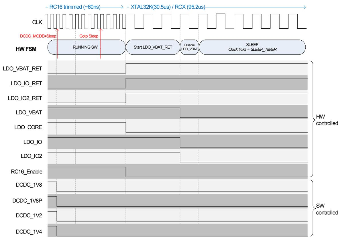
Figure 17: Goto Sleep timing and PMU operations
