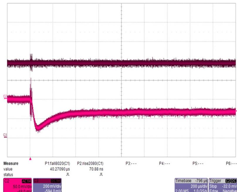
Figure 15: LDO\_VBAT\_RET loadstep 0 to 5mA (Cload=4.7uF, Vout=2.4V)
