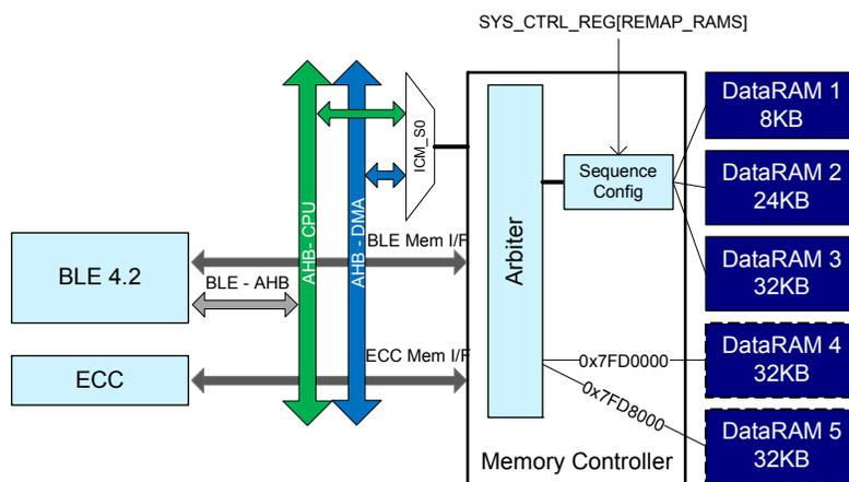
Figure 34: Memory Controller Block Diagram and environment
