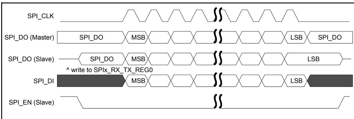
Figure 74: SPI Master/Slave, mode 1: SPI\_POL=0 and SPI\_PHA=1
