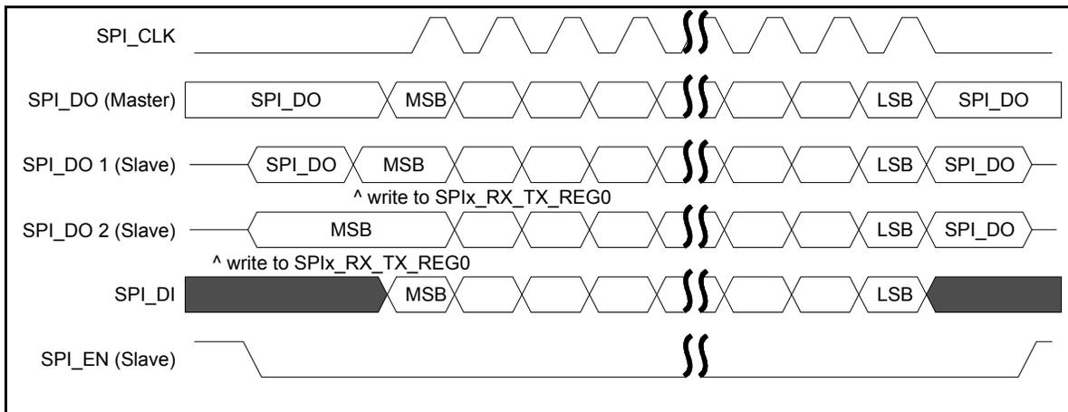
Figure 73: SPI Master/slave, mode 0: SPI\_POL=0 and SPI\_PHA=0
