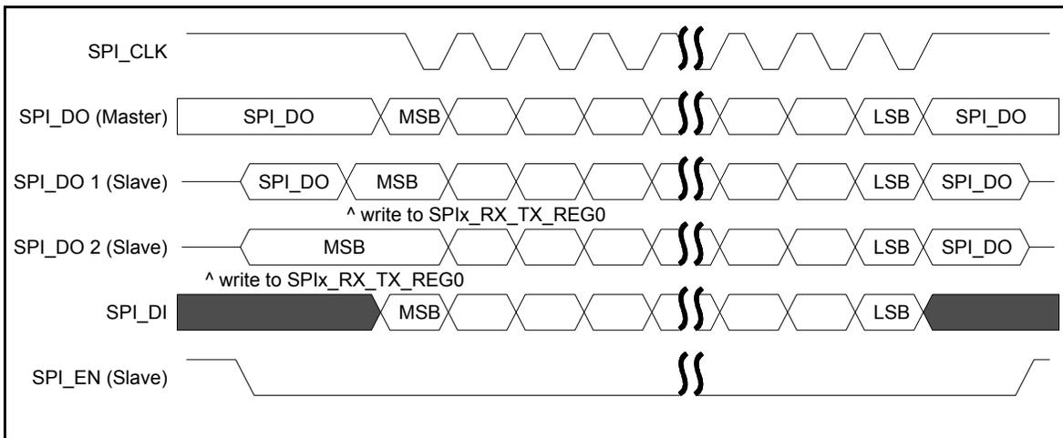
Figure 75: SPI Master/Slave, mode 2: SPI\_POL=1 and SPI\_PHA=0
