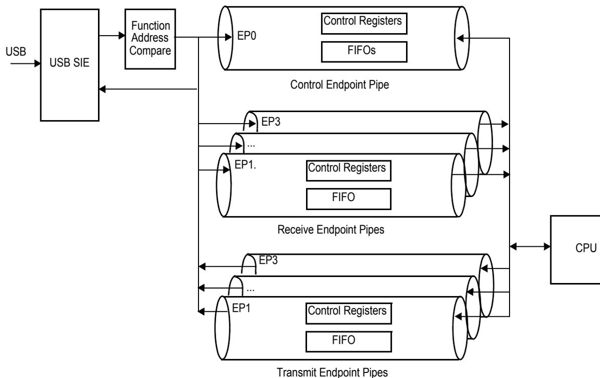
Figure 104: Endpoint Operation
