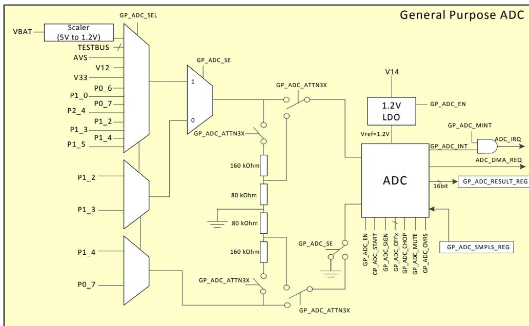
Figure 53: Block diagram of the General Purpose ADC
