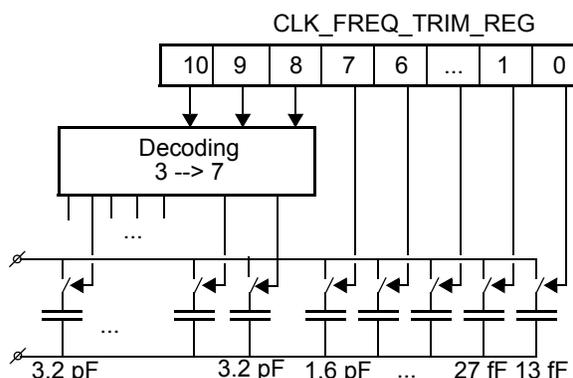
Figure 28: Frequency trimming
