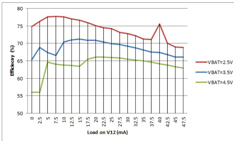
Figure 11: 1.2V rail DCDC efficiency vs load
