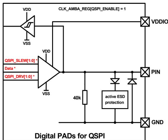
**Figure 113: Latching of QSPI pad signals**
