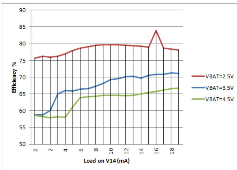
Figure 12: 1.4V rail DCDC efficiency vs load
