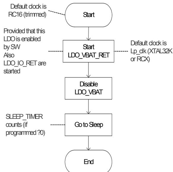
**Figure 4: Go to Sleep FSM flow diagram**
