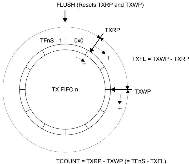
**Figure 108: Tx FIFO operation**
