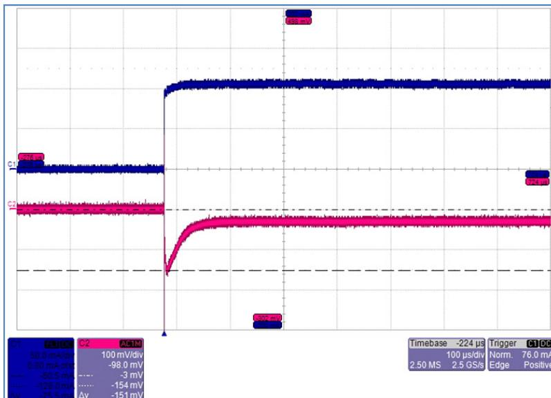
Figure 13: LDO\_VBAT loadstep 0 to 100mA (Cload=4.7uF, Vout=3.3V)
