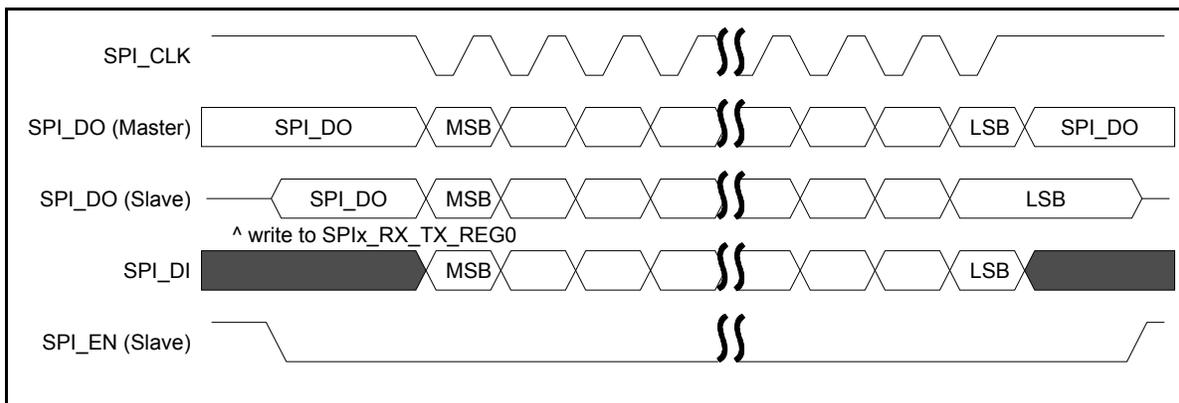
Figure 76: SPI Master/slave, mode 3: SPI\_POL=1 and SPI\_PHA=1
