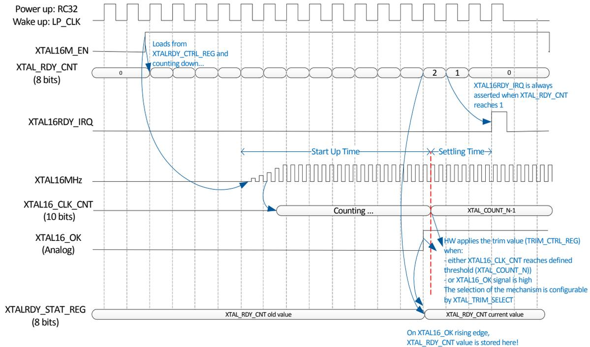
**Figure 29: Automated mechanism for XTAL16M trim and settling**
