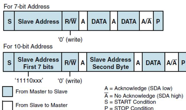
Figure 84: Master-Transmitter Protocol
