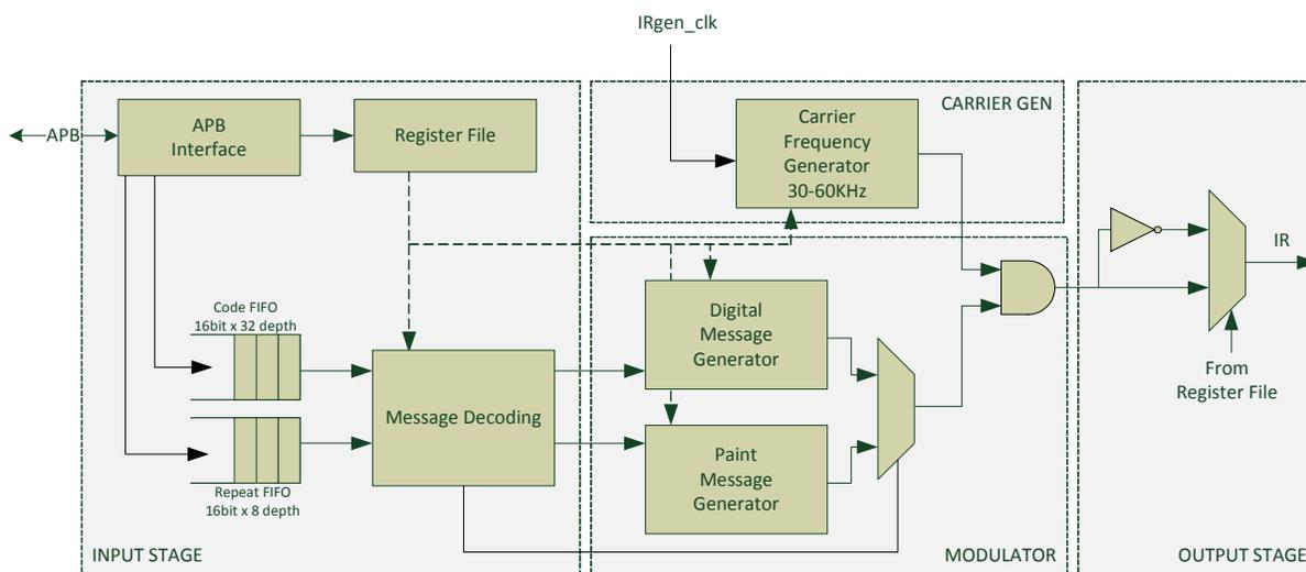
Figure 89: InfraRed Generator Block Diagram
