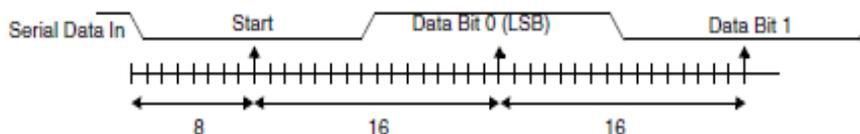
Figure 68: Receiver Serial Data Sample Points
