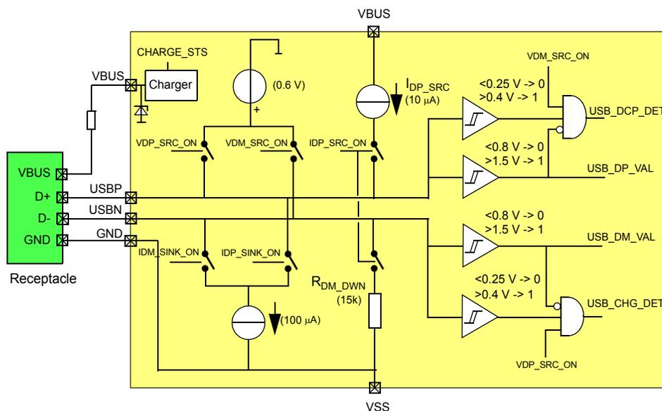
Figure 24: USB charger detection block diagram (BC1.2)
