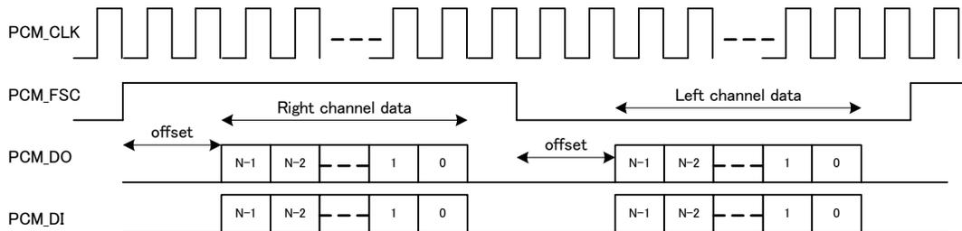
**Figure 64: I2S TDM mode (left justified mode)**
