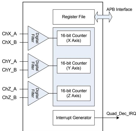
Figure 91: Block diagram of the Quadrature Decoder
