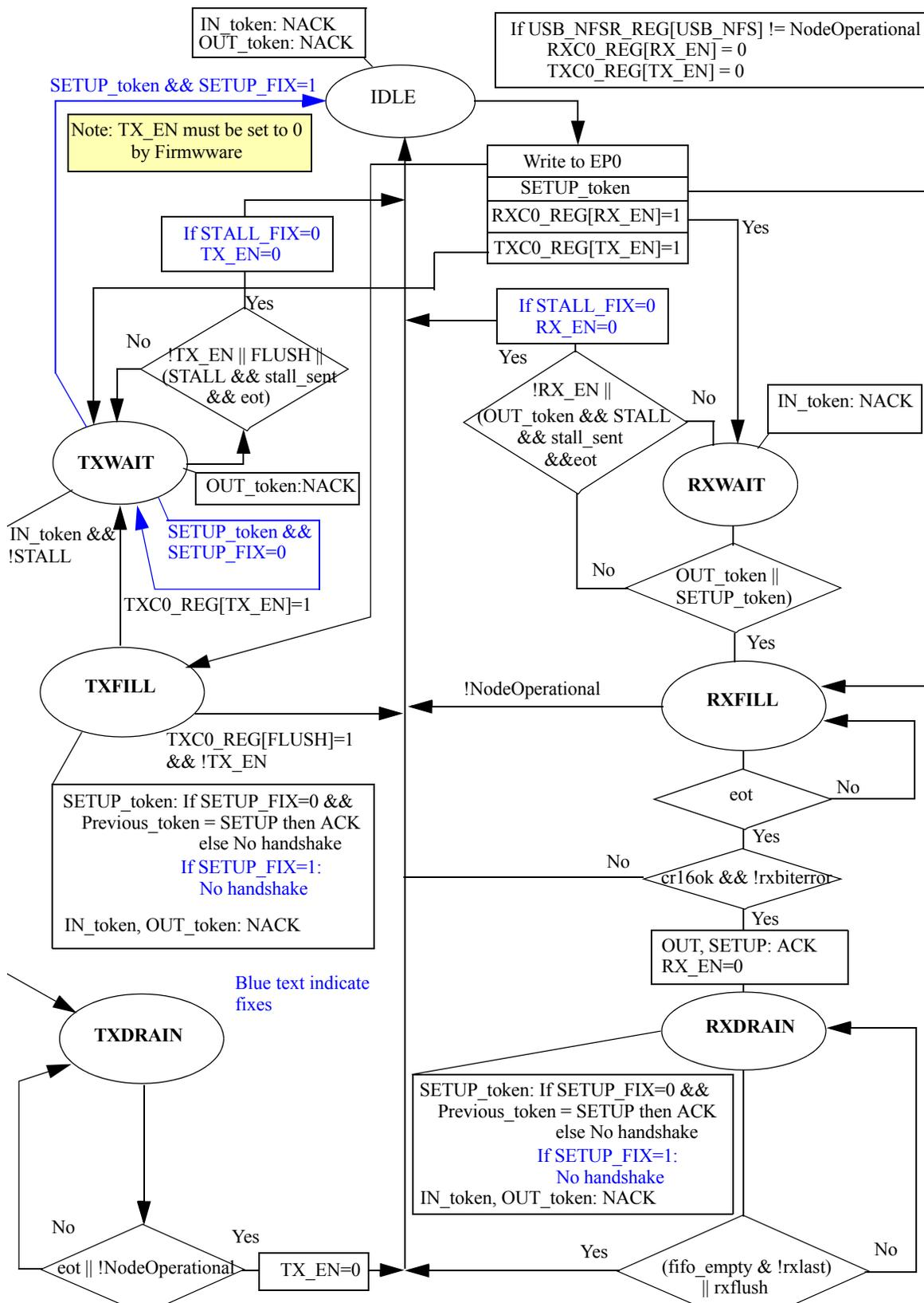
Figure 107: Endpoint 0 Operation
