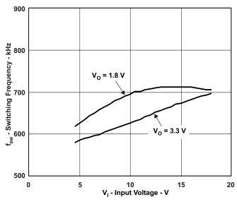
Figure 9. SWITCHING FREQUENCY vs INPUT VOLTAGE
