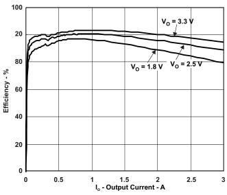
Figure 7. EFFICIENCY vs. OUTPUT CURRENT  $(V_{IN} = 12 V)$
