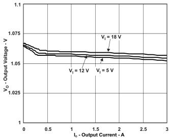
Figure 3. 1.05-V OUTPUT VOLTAGE vs. OUTPUT CURRENT
