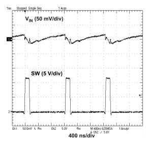
Figure 12. VOLTAGE RIPPLE At INPUT
