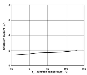
Figure 2. V<sub>CC</sub> SHUTDOWN CURRENT vs. JUNCTION TEMPERATURE
