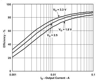
Figure 8. LIGHT LOAD EFFICIENCY vs. OUTPUT CURRENT
