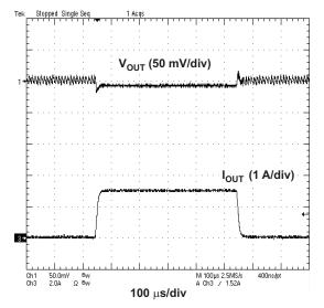
Figure 5. 1.05-V, 0-A TO 3-A LOAD TRANSIERESPONSE
