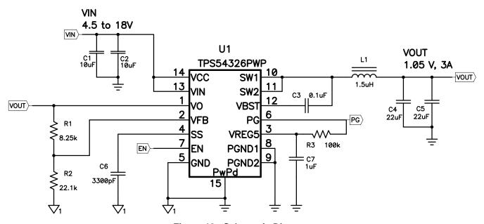
Figure 13. Schematic Diagram
