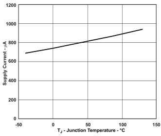
Figure 1. V<sub>CC</sub> SUPPLY CURRENT vs. JUNCTION TEMPERATURE
