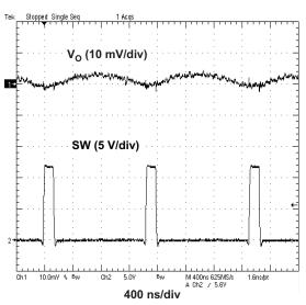
Figure 11. VOLTAGE RIPPLE At OUTPUT
