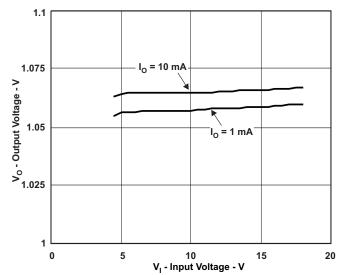
Figure 4. 1.05-V OUTPUT VOLTAGE vs. INPUT VOLTAGE
