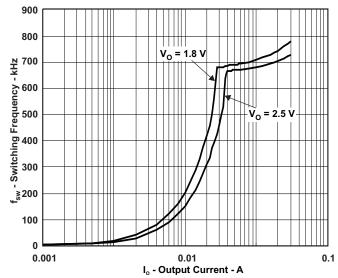
Figure 10. SWITCHING FREQUENCY vs OUTPUT CURRENT
