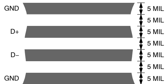
Figure 34. Typical Arrangement of Signal Tracks
