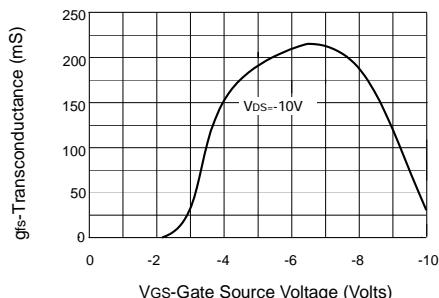
**Transconductance v gate-source voltage**
