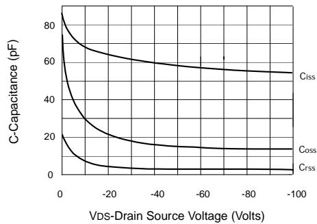
**Capacitance v drain-source voltage**
