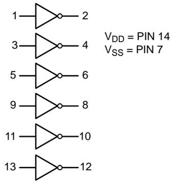
Figure 1. Logic Diagram
