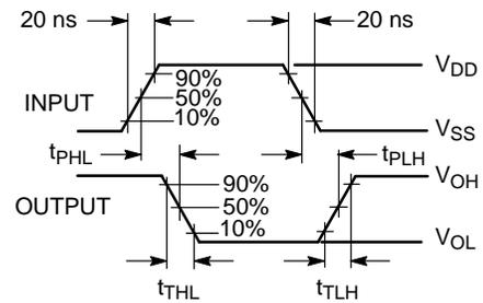
Figure 3. Switching Time Test Circuit and Waveforms
