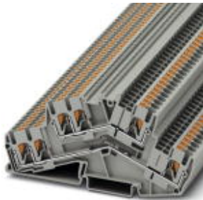
Double-level terminal block, Cross section: 0.14 mm 2 - 4 mm 2 , AWG: 26 - 12, Connection type: Push-in connection, Width: 5.2 mm, Color: gray, Mounting type: NS 35/7,5, NS 35/15
