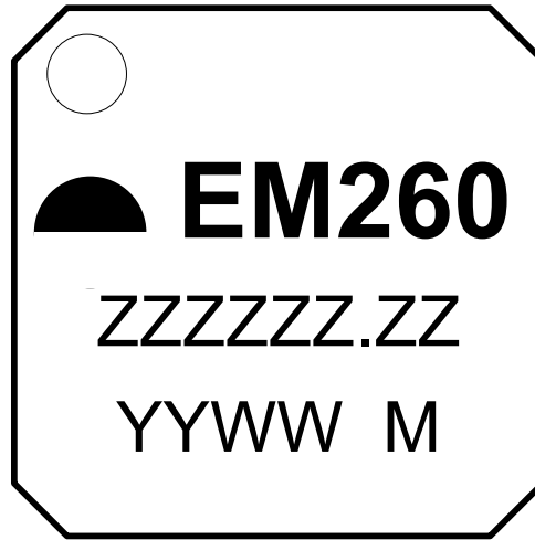
Figure 22. Part marking for EM260
