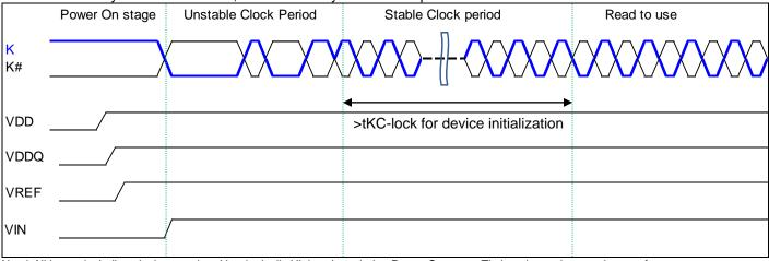
Note) All inputs including clocks must be either logically High or Low during Power On stage. Timing above shows only one of cases.
