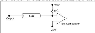
(b) tCHQZ and tCHQX1 are specified with 5pF load capacitance and measured when transition occurs ±100mV from
