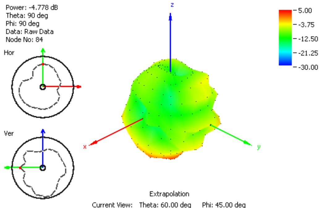
**Figure 11.** Radiation pattern at 900 MHz, Figure 1 as reference (dB), with 2m RG174 cable and free space.
