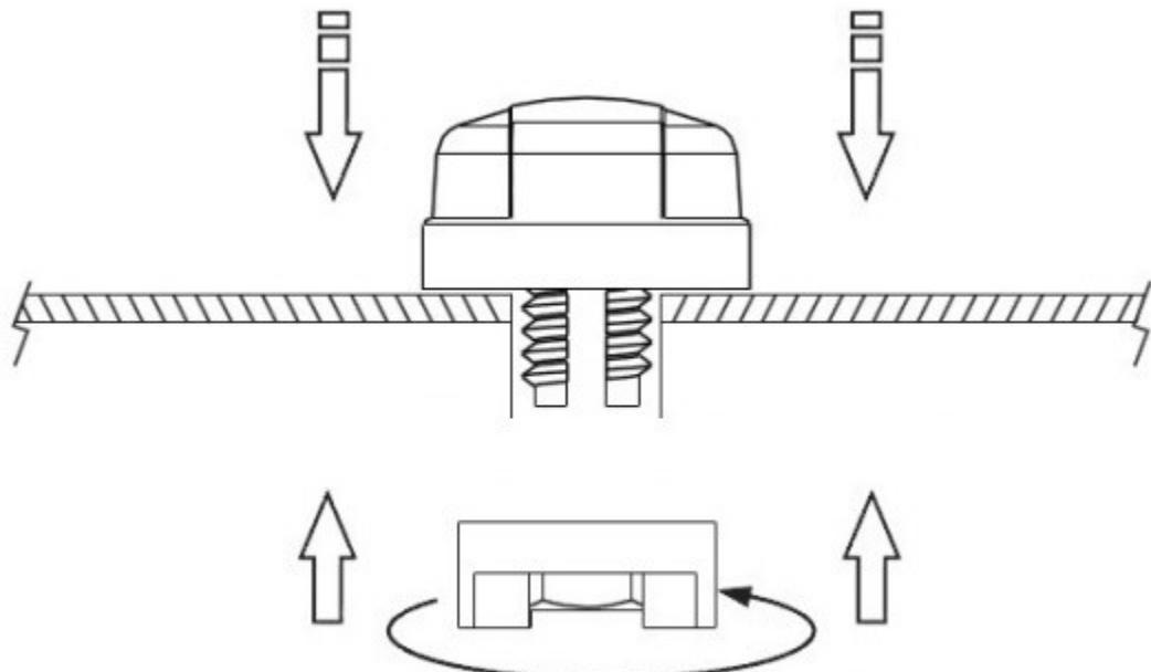
Recommended torque for Mounting is 24.5N·m
