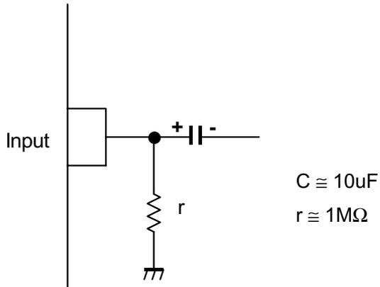
This IC requires  $0.1\mu\text{F}$  capacitor between INPUT and GND,  $1\text{M}\Omega$  resistance between INPUT and GND for clamp type input at mute mode.
