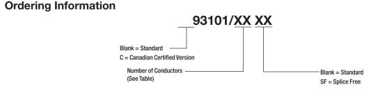
Note: Available in standard 100 ft rolls. Contact 3M for availability of additional conductor counts and/or custom roll lengths.
