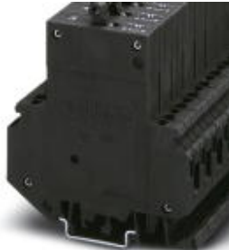
Thermomagnetic circuit breaker, 1-pos., normal blow, 1 N/O contact, with universal foot for mounting on NS 32 or NS 35
