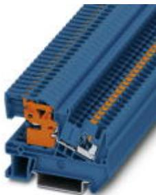
N disconnect terminal block, Push-in connection, Cross section: 0.14 mm<sup>2</sup> - 4 mm<sup>2</sup>, AWG: 26 - 12, Width: 5.2 mm, Color: blue, Mounting type: NS 35/7,5, NS 35/15
