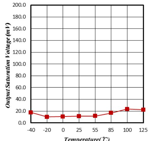
Figure 6. Output Saturation Voltage vs. Temperature
