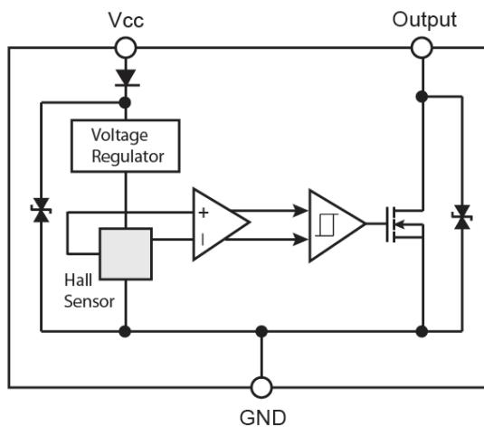
**Note:** Static sensitive device; please observe ESD precautions. Reverse VDD protection is not included. For reverse voltage protection, a 100Ω resistor in series with VDD is recommended.
