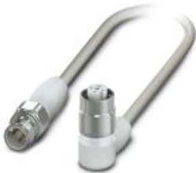
Sensor/Actuator cable, 4-position, PP-EPDM halogen-free, Gray RAL 7035, Plug straight M12, A-coded, on Socket angled M12, A-coded, Cable length: 0.6 m, Hygienic design, With high-grade steel knurl
