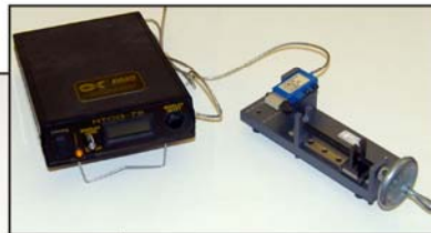
RTCG-75 Retention Tester Calibration Gage
