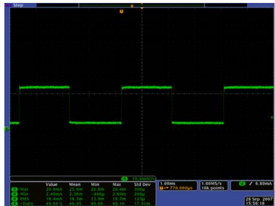
FIGURE 16. I LED AT 50% PWM DIMMING
