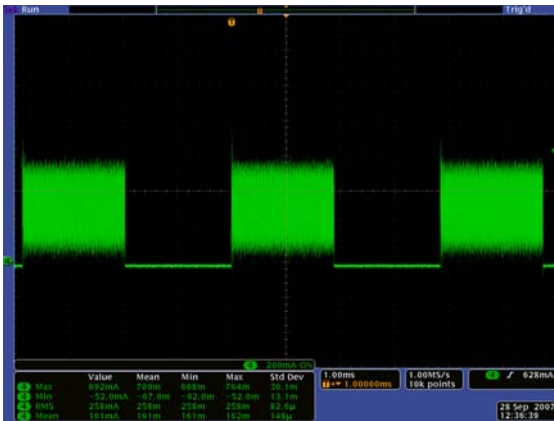
FIGURE 11. IL AT 50% PWM DIMMING
