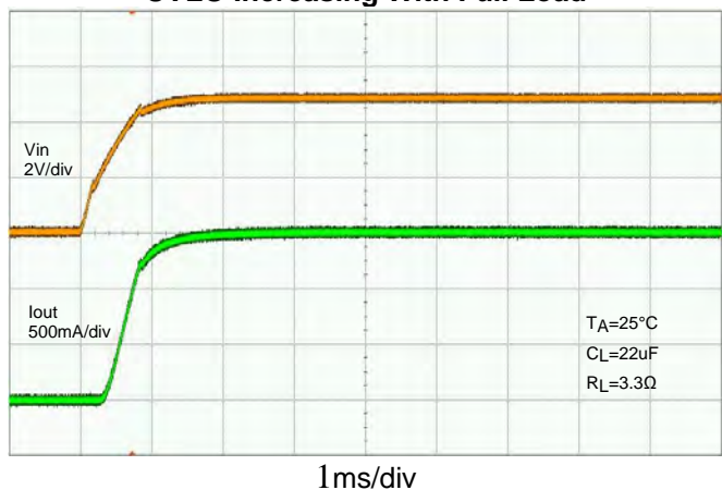
UVLO Increasing With Full Load
