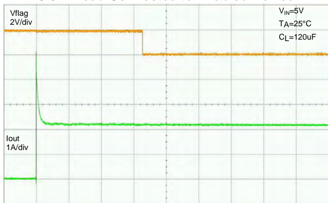
0.6 Ω Load Connected to Enabled Device
