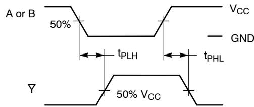
Figure 3. Switching Waveforms
