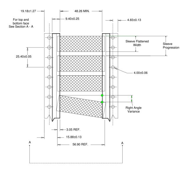
Figure 1: Assembly schematic of TMS-90-SCE
