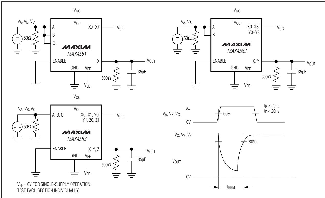
Figure 4. Break-Before-Make Interval
