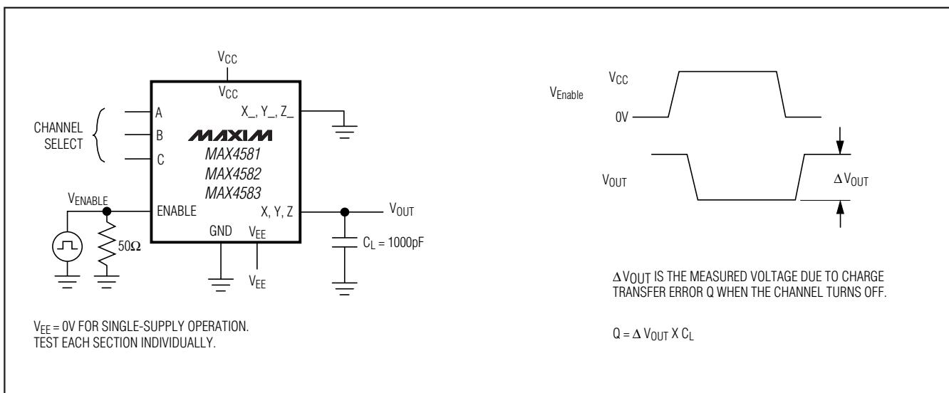
Figure 5. Charge Injection
