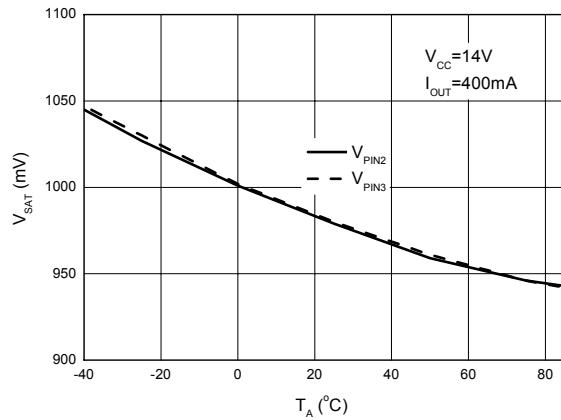
Figure 12. V<sub>SAT</sub> vs. Ambient Temperature
