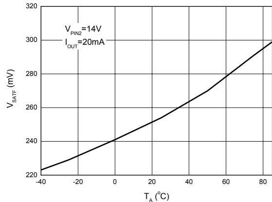
Figure 14. FG Saturation Voltage vs. Ambient Temperature
