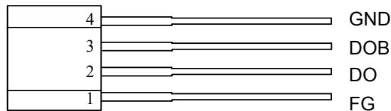
Figure 2. Pin Configuration of AH211 (Front View)
