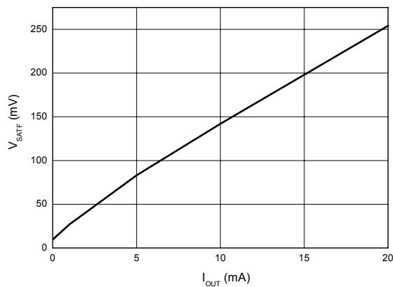
Figure 13. FG Saturation Voltage vs. Output Current
