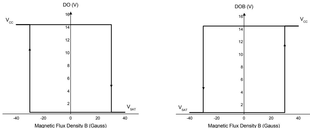
Figure 5.  $V_{DO}$  vs. Magnetic Flux Density
