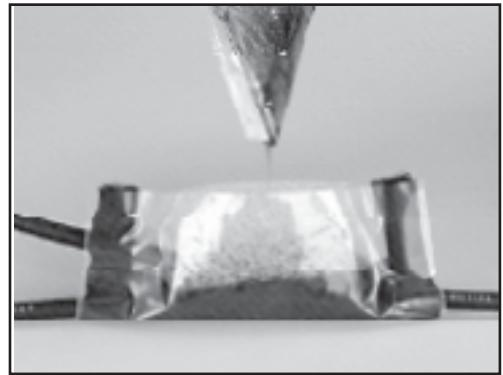
**3.10 Seal Top of Mold.** Remove liner from adhesive film strip supplied with kit. Tape it over the mold leaving a loop over mold opening.
