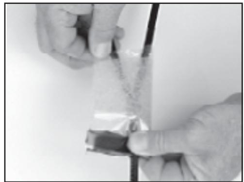
**4.5** Remove liner from adhesive film strip supplied with kit.
