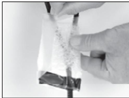
**4.7** Mix the resin per instructions on resin package. Pour into mold.
