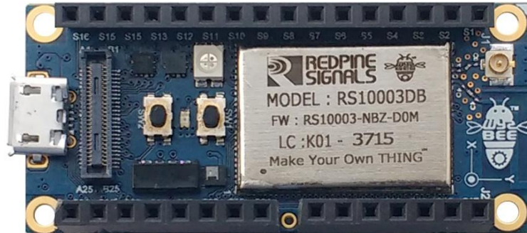
Figure 2: WyzBee™ Baseboard's Top View
