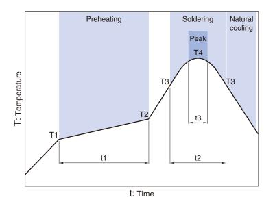
Preheating Soldering Peak Temp. Temp. Temp. Time Time Time T1 T2 t1 ТЗ t2 **T4** t3 150°C 180°C 60 to 120s 230°C 30 to 50s 250 to 260°C 10s max.
