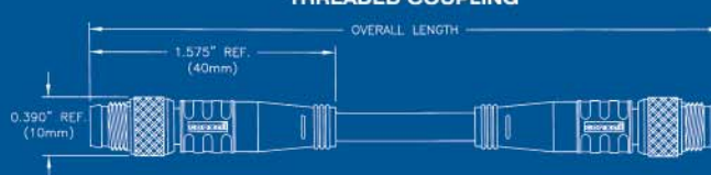
STRAIGHT/90° MALE/FEMALE DOUBLE ENDED THREADED COUPLING
