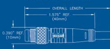
STRAIGHT FEMALE SINGLE ENDED THREADED COUPLING
