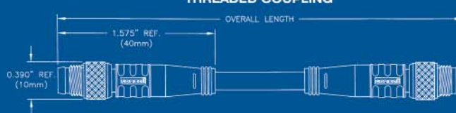
STRAIGHT/90° MALE/FEMALE DOUBLE ENDED THREADED COUPLING
