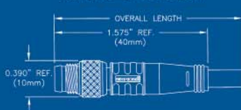
STRAIGHT FEMALE SINGLE ENDED THREADED COUPLING
