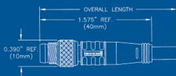
STRAIGHT FEMALE SINGLE ENDED THREADED COUPLING
