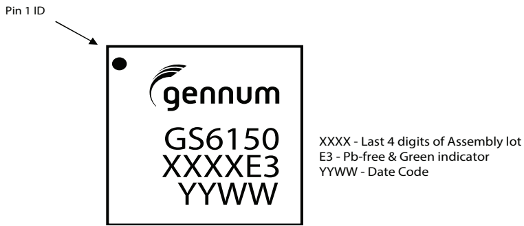
Figure 7-3: GS6150 Marking Diagram
