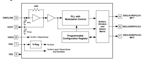
\*MF: Programmable input control pin as PD#, OE, SSON# (Spread On/Off) or FSEL (Frequency Select)
