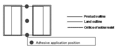
Amount of adhesive applied is a standard 1/2 to 2/3 of the bottom flange thickness.
